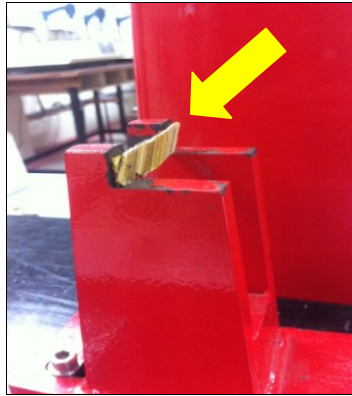
Figure 7: Charpy test configuration
