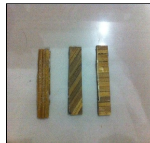
Figure 6: Specimen of 0^{\circ} , 60^{\circ} & 90^{\circ}
