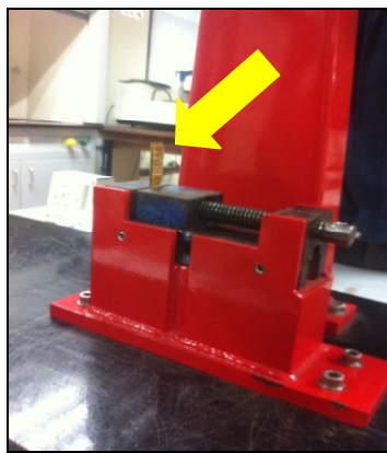
Figure 8: Izod test configuration
